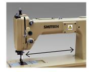
Extended arm (400 mm) to fit thick and long materials under the sewing machine.
