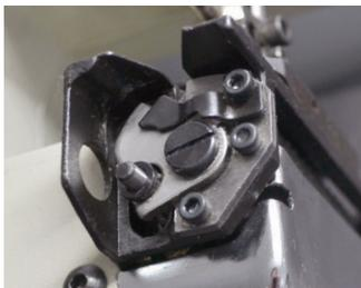
Integrated thread cutter to cut the thread after sewing.
