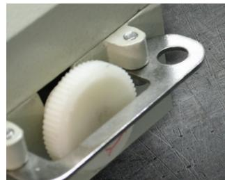
Attachement hole for connecting a hook, spring balancer or other equipment to hang the Smitsen UP2 safely from the back.
